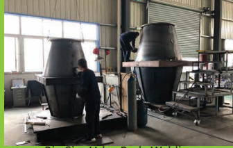
Big Size Valve Body Welding
